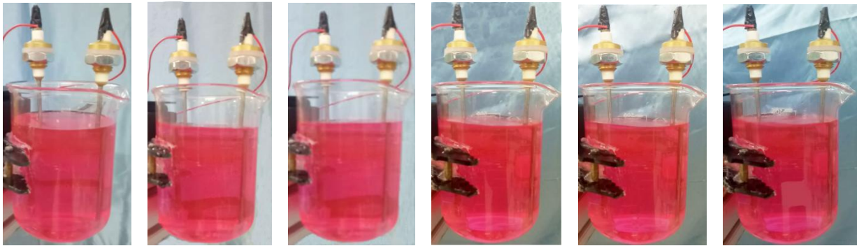
Fig.16 Simulation and experimental results of liquid sloshing at \delta=0.5
