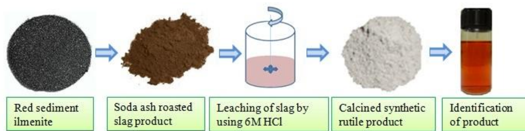
Fig 11. Graphical representation of leaching kinetics of soda ash roasted slag of red sediment ilmenite for production of synthetic rutile [15]
