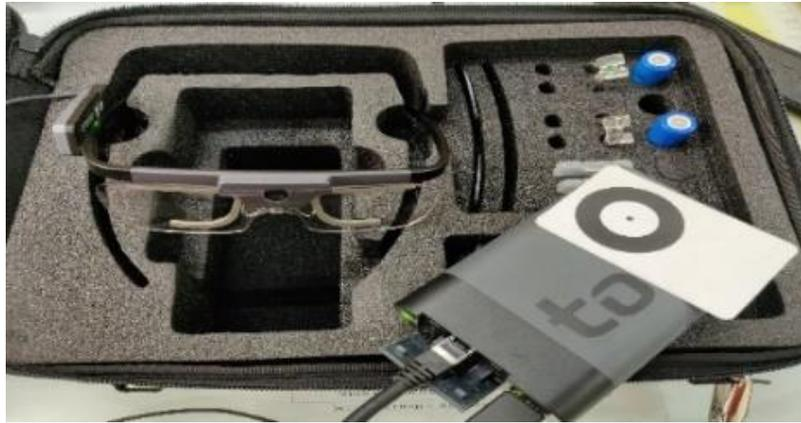
**Figure 1 Wearable Tobii Glass Eye Tracker**
