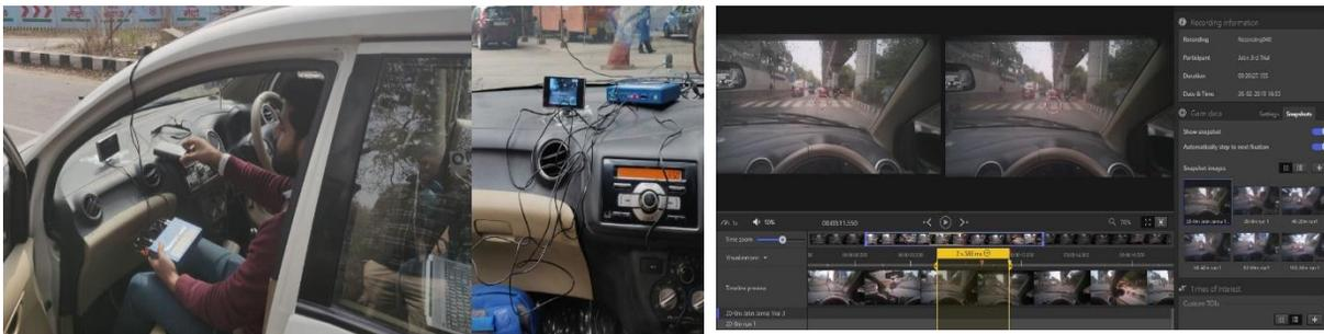
**Figure 2: Setup of V-Box and Eye tracker Software with timeline data series.**
