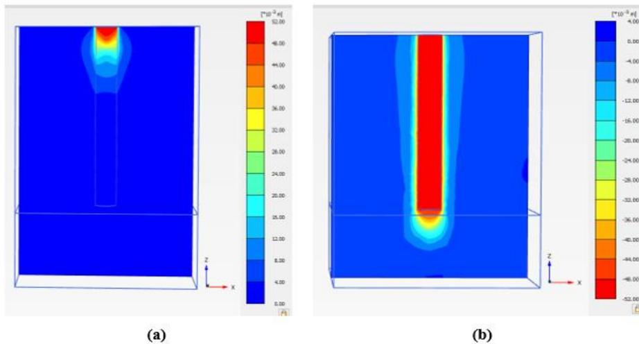
**Figure 8.** Shadings of vertical displacements: (a) SC; (b) PCC.
