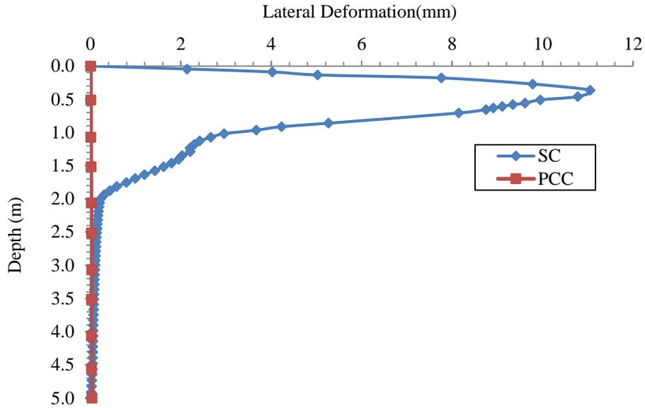
**Figure 7.** Lateral deformation of column along the length.
