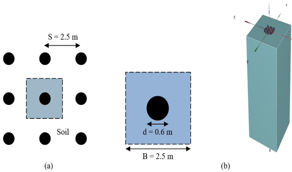
**Figure 1.** Three-dimensional column: (a) column layout; (b) 3 D column.
