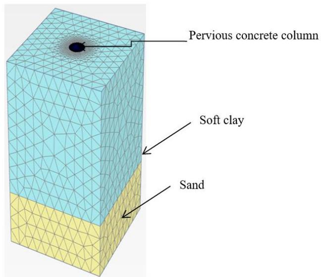
**Figure 2.** Three-dimensional model of the column.
