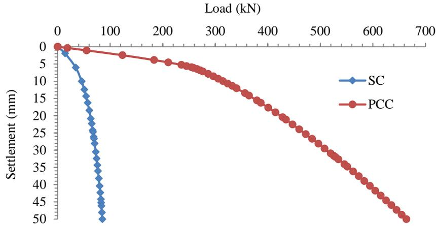
**Figure 5.** Load-settlement behavior of a SC and PCC.
