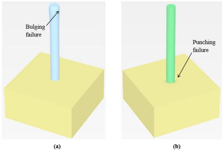
**Figure 6.** Deformed shapes: (a) SC; (b) PCC.
