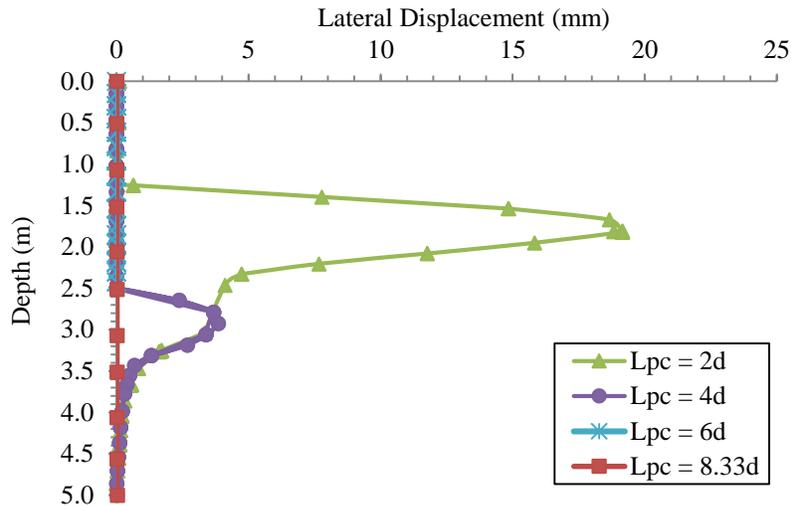
**Figure 11.** Lateral deformation vs. depth at a vertical stress of 625 kPa for a CC, and PCC with varying length of pervious concrete.
