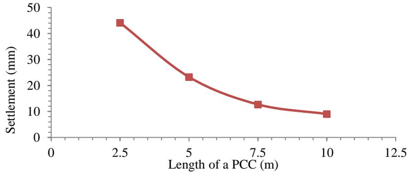
**Figure 13.** Settlement at a vertical load of 450 kN for different length of a PCC.
