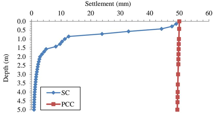
**Figure 9.** Vertical settlement vs. depth of column.
