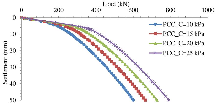
**Figure 15.** Load vs. settlement of PCCs at 50 mm vertical settlement considering different values of cohesion.
