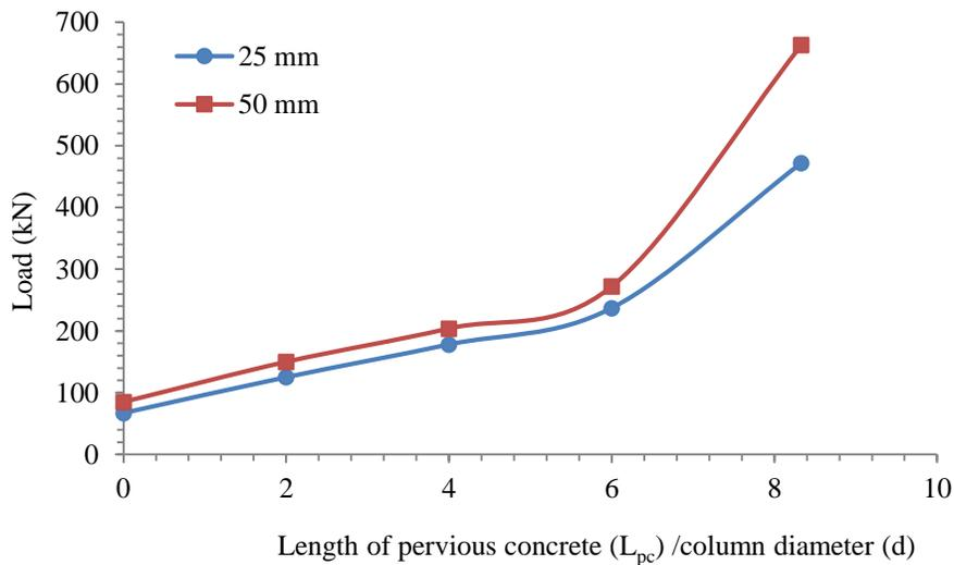
**Figure 10.** Mobilized vertical load in a SC, PCC, and CC as a function of  $L_{pc}$ .
