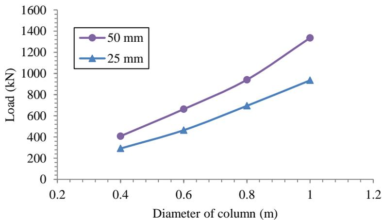
**Figure 12.** Load vs. diameter of a PCC for a settlement of 25 and 50 mm.
