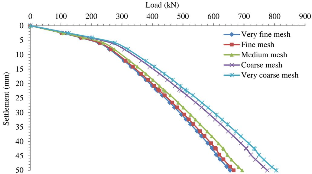
**Figure 3.** Convergence study for determining the optimum mesh size.
