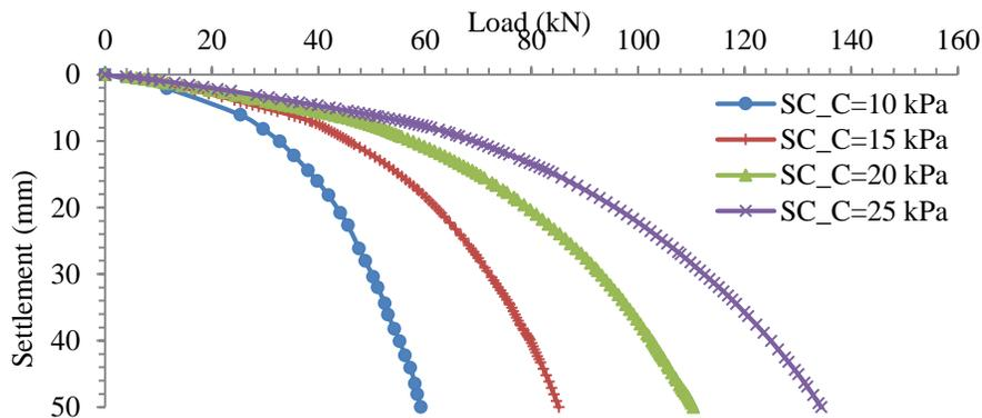
**Figure 14.** Load vs. settlement of SCs at 50 mm vertical settlement considering different values of cohesion.
