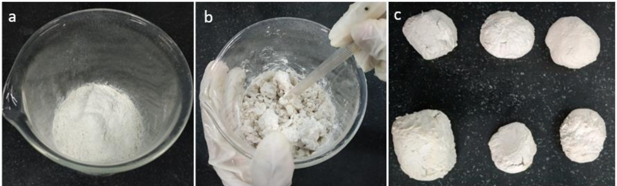
494 Figure 1. Steps followed in the process of poulting (a) cellulose powder in the dry form (b) 495 mixing of cellulose powder with water to prepare the poultrice (c) samples covered with the 496 cellulose poultrice left for drying
