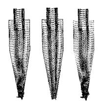
for each cyclone. Fluid mixture enters the cyclone and makes a double-swirl motion and the dense phase of the mixture is separated from the main flow by the centrifugal forces. It is difficult to analyse this problem since, in addition to its 3D character, there are many parameters influenced this flow. Therefore, this complex swirling turbulent flow in a cyclone requires efficient numerical techni-
