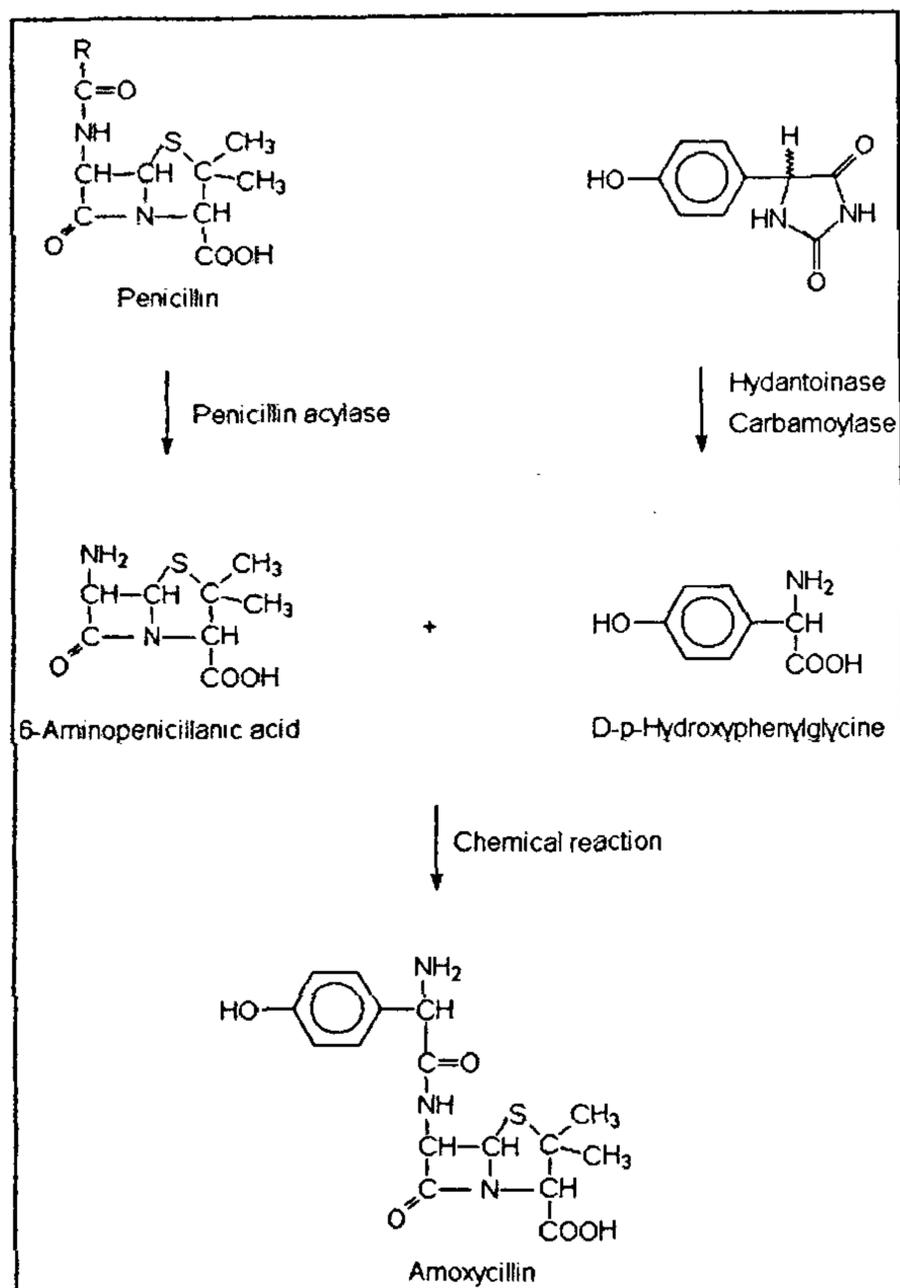
Figure 1. Schematic representation of amoxicillin production.
