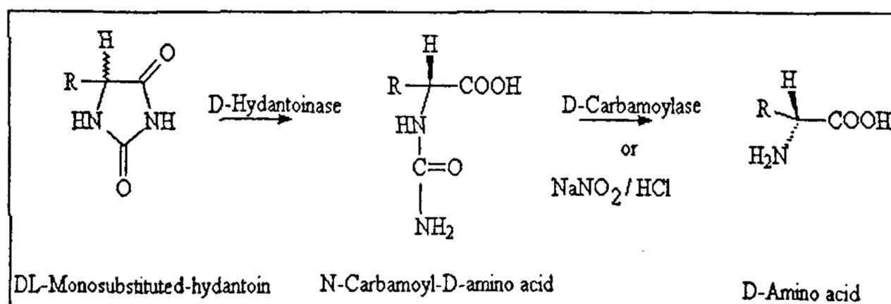
Figure 2. Schematic representation of hydantoinase/carbamoylase process for the production of D-amino acids.
