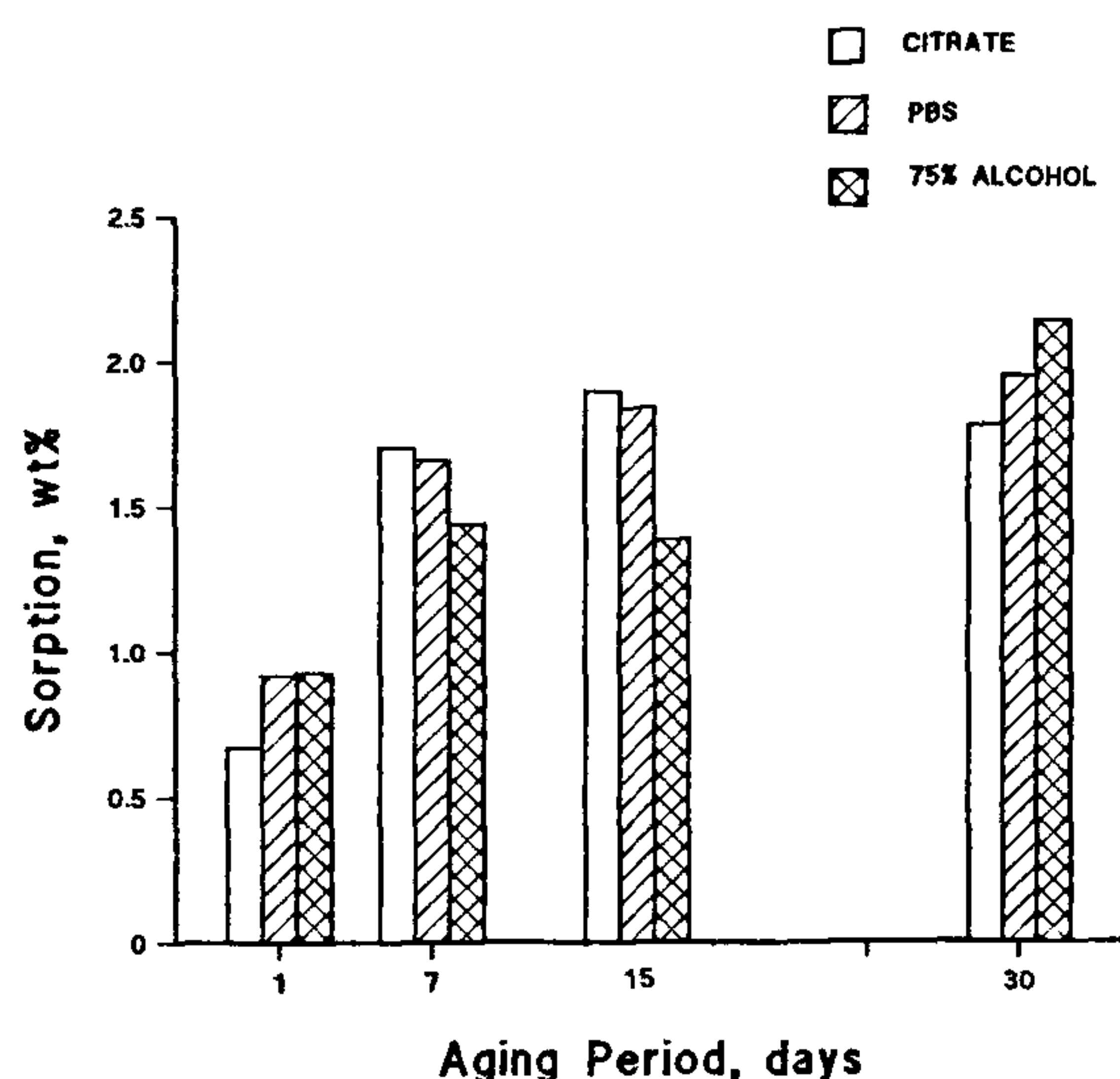
Figure 2. Sorption changes with ageing time in three media for urethane dental composite.
