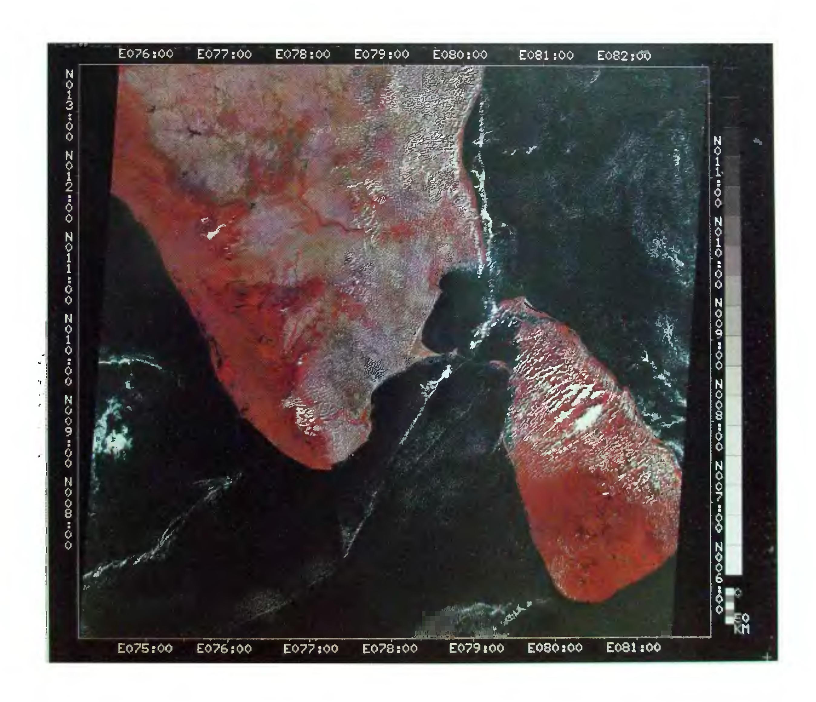
The Wide Field Sensor (WiFS) operates in visible and near IR region with a spatial resolution of 188 m and a swath of 810 km. Because of the wide swath the camera can observe the same region once in every 5 days. The figure shows the WiFS image acquired soon after the launch covering South India and Srl Lanka. The red colour indicates vegetation and pure white patches are clouds. Reservoir and river courses are also seen.
