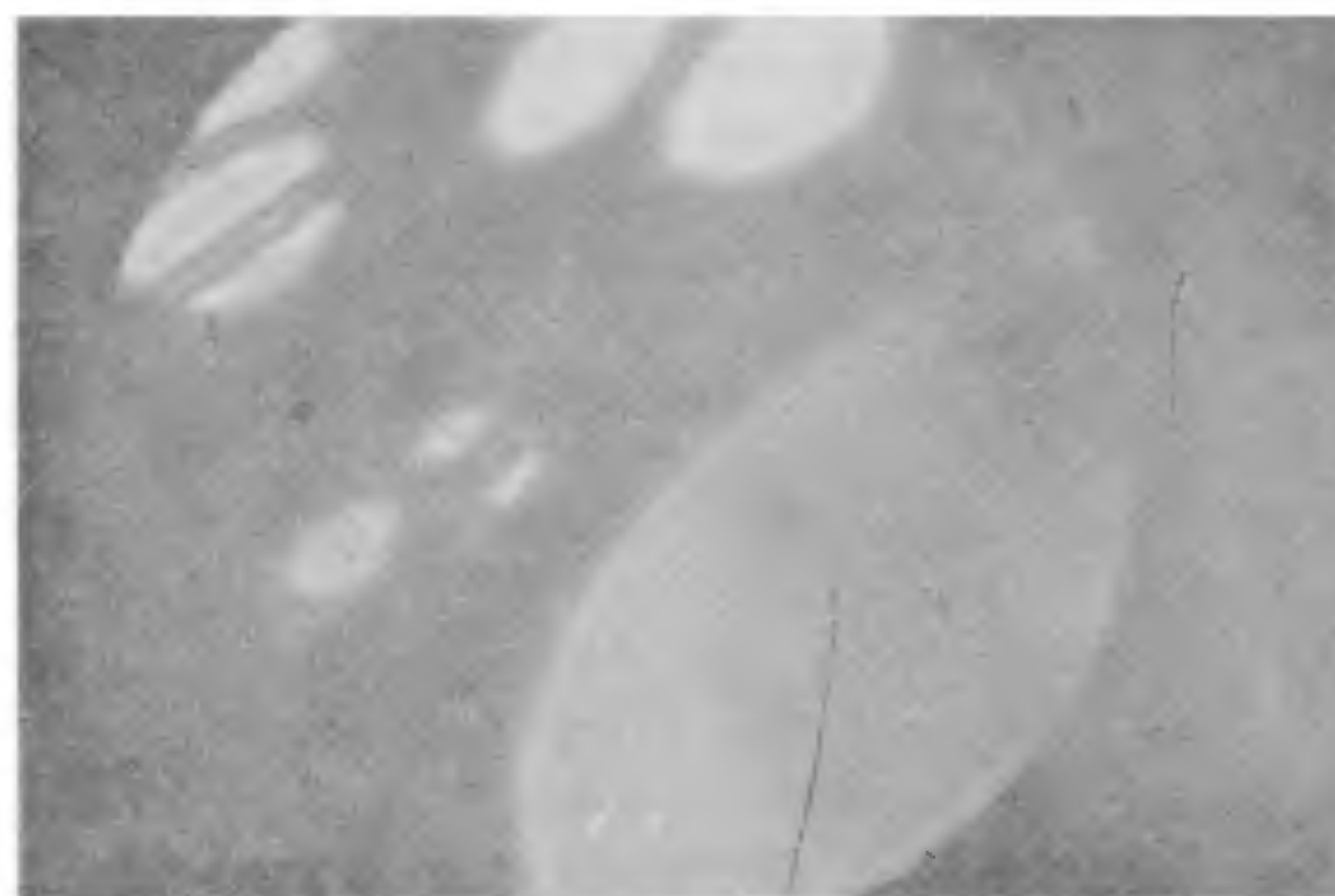
Figure 5. Projection image of a perforated carbon film recorded with 90 eV electrons for Z_1 = 461 nm and Z_2 = 14 cm, leading to a magnification of 304 000. An intensity trace across the Fresnel fringes allows one to determine the size of the source and its brightness and coherence parameters of the beam.
