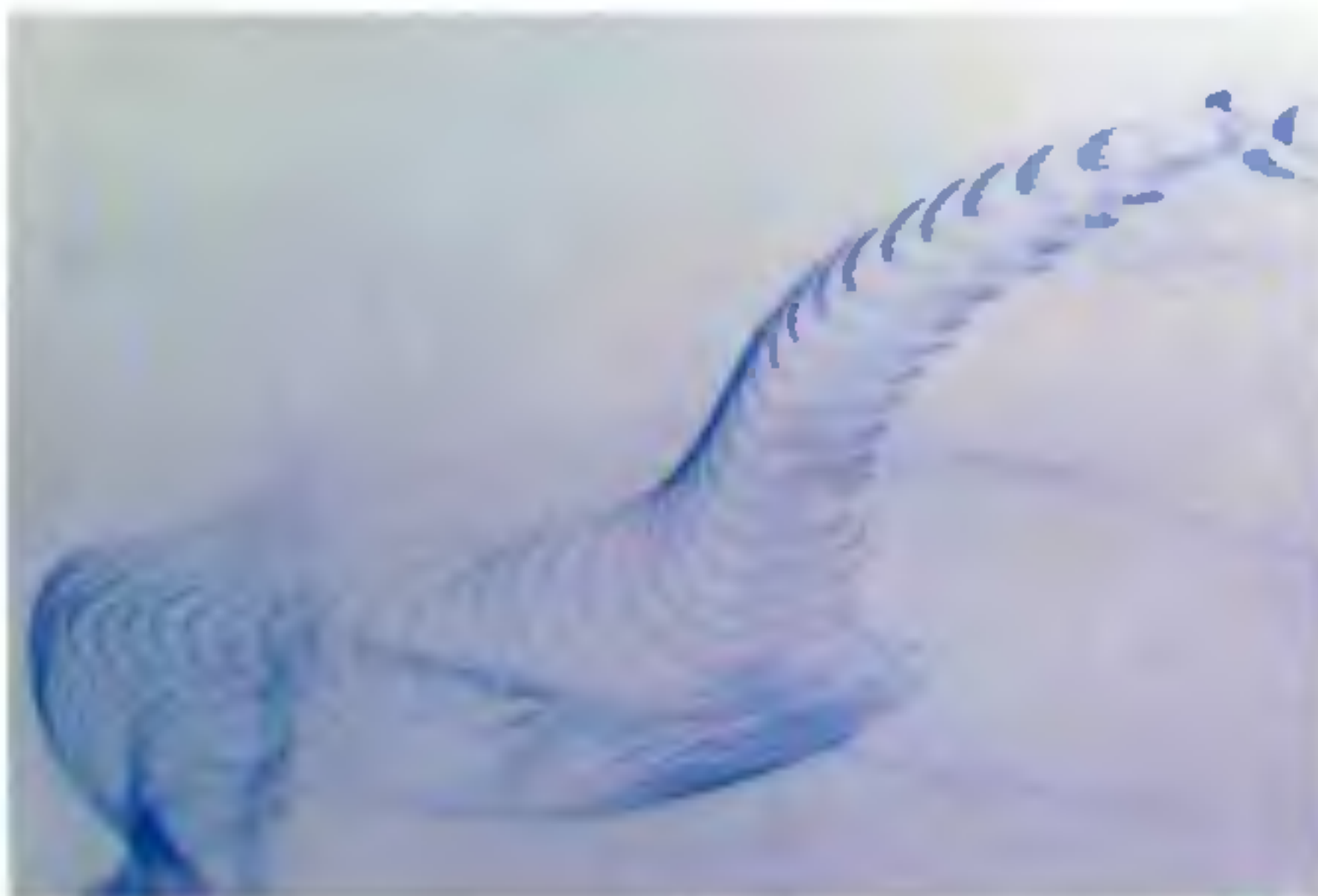
Figure 7. A pattern generated when successive drops are released and the resulting vortices are allowed to be influenced by convection currents or wakes in the pool
