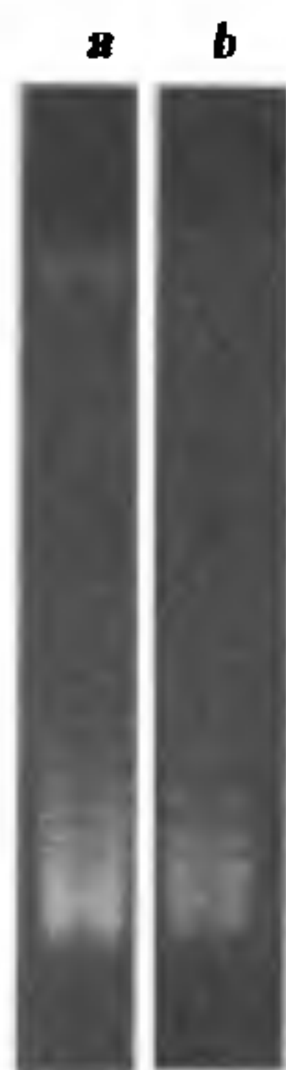
Figure 3. Analysis of topoisomers on 1% agarose gel in the presence of a and b , panels a and b respectively, Supercoiled pBR322 plasmid DNA was analysed in the presence of 2 \mu\text{g ml}^{-1} of intercalator in TBE buffer.
