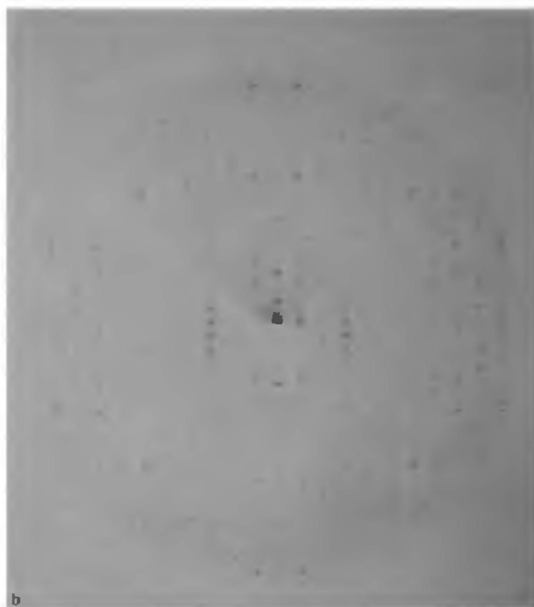
Figure 1. okl 15^\circ precession photographs from the new crystal form of ribonuclease A at (a) 100% and (b) 90% relative humidity.
