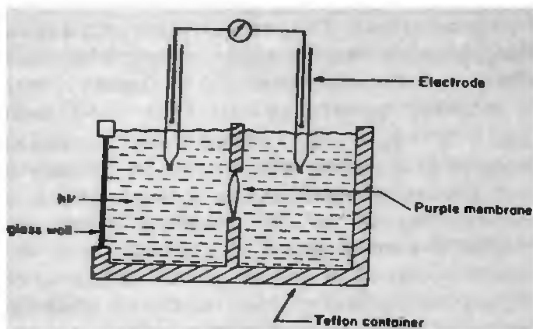
**Figure 2.** Photoelectrochemical cell.
