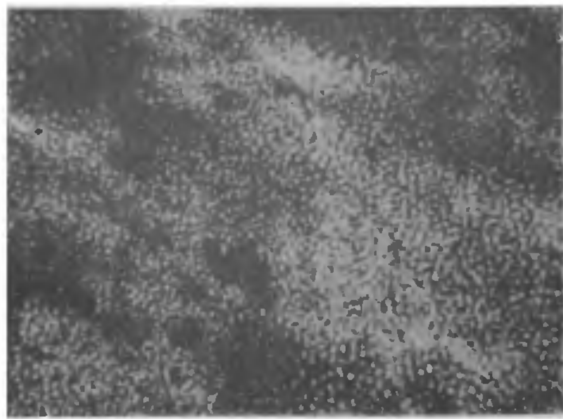
Figure 2 Etch pattern obtained for Al-Zn system at the beginning of oxidation ( \times 120 ) (etchant used: alcoholic solution of sodium hydroxide).
