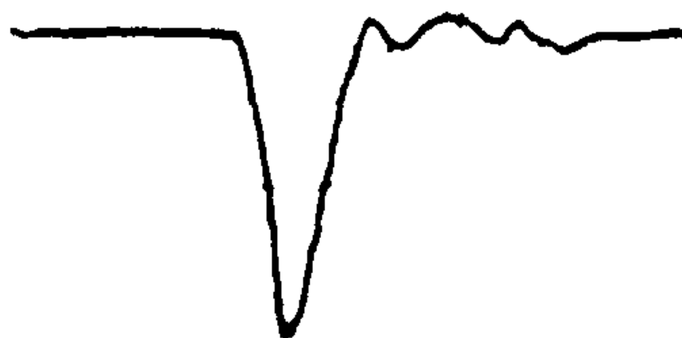
FIG. 2. Output pulse of the discriminator. Pulse rise time 10 ns \text{cm}^{-1} ; pulse height 1 V \text{cm}^{-1} .
