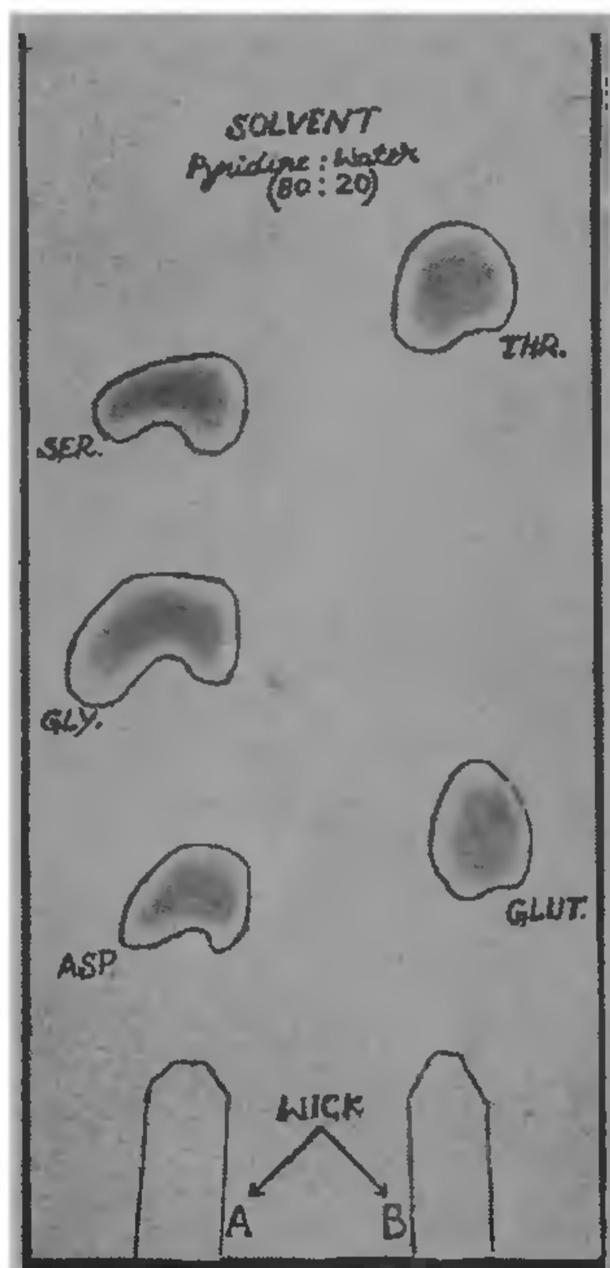
FIG. 2. Ascending Paper chromatogram No. 2 in Pyridine: Water, showing separation of the five amino-acids.
