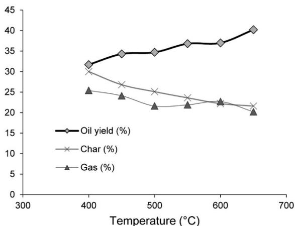
**Figure 1.** Product distribution from batch pyrolysis of pine needles.
