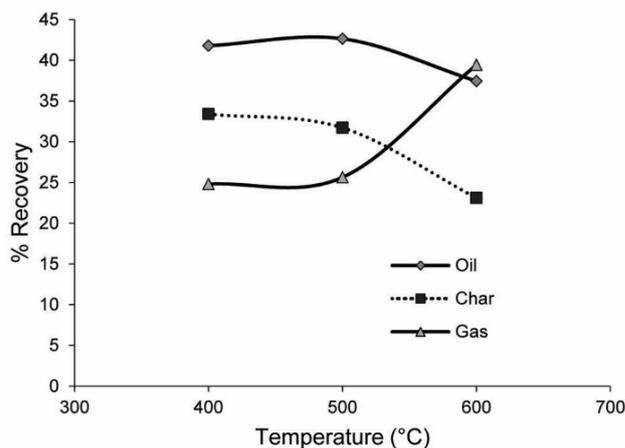
**Figure 2.** Product distribution from continuous pyrolysis of pine needles.
