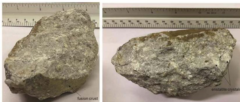
**Figure 3.** Meteorite sample in hand specimen. (Left) Light brown fusion crust is visible. (Right) Large enstatitic pyroxene grains occurring as bright white crystals. Scale is in inches.
