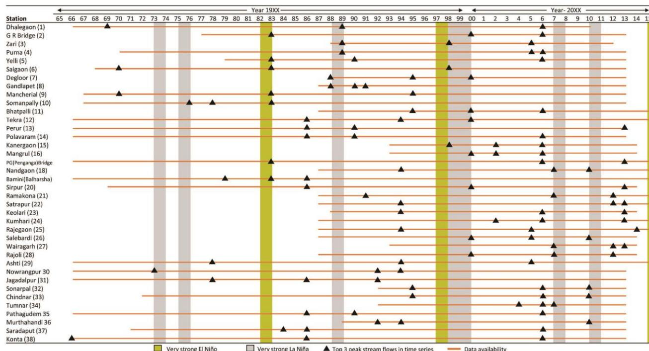
**Figure 1.** Station-wise data range. The top three peak streamflow years have been plotted for each station to determine the most severe flood years (e.g. the 2006 flood had led to extreme discharge in almost the entire catchment). Very strong El Niño and La Niña years have been determined based on NOAA data ([https://origin.cpc.ncep.noaa.gov/products/analysis\\_monitoring/ensostuff/ONI\\_v5.php](https://origin.cpc.ncep.noaa.gov/products/analysis_monitoring/ensostuff/ONI_v5.php)).
