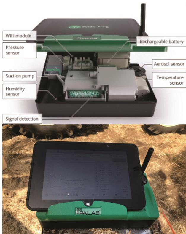
**Figure 2.** Real-time dust sampler (Fidas® Frog fine dust monitoring device).
