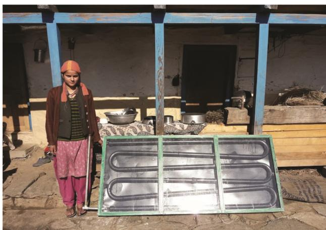
**Figure 1.** Mountain solar water-heating system in a rural household.
