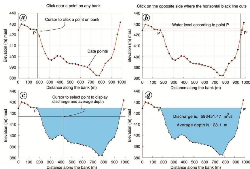
**Figure 1.** Channel cross-sections generated at different steps of the tool. *a*, Cross-section profile generated after import of data; *b*, With water stage after first click; *c*, Water inundated shown by shaded region; *d*, Final display with values of water discharge and average depth.
