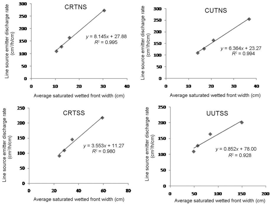
Figure 3. Variation of saturated wetted front width for surface line-source drippers.
