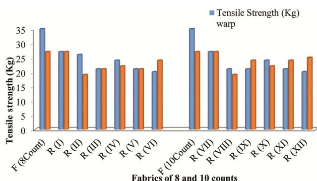
**Figure 1.** Tensile strength of 8 and 10 counts fresh and recycled fabrics. F, Fresh/control fabrics; R, Recycled fabrics.
