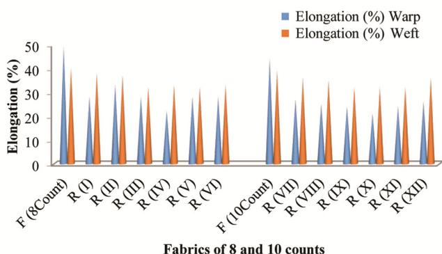
**Figure 2.** Elongation of 8 and 10 counts fresh and recycled fabrics. F, Fresh/control fabrics; R, Recycled fabrics.
