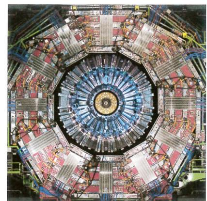
Transverse section of the barrel part of CMS, illustrating the successive layers of detection starting from the centre, where the collisions occur: the inner tracker, the crystal calorimeter, the hadron calorimeter, the superconducting coil, and the iron yoke instrumented with the four muon stations. The last muon station is at a radius of 7.4 m.
