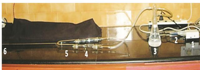
**Figure 1.** Y-tube olfactometer used in the bioassay: 1, Air pump; 2, Charcoal filter; 3, Humidifier; 4, Sample/control arm; 5, Y-tube; 6, Weevil release point.
