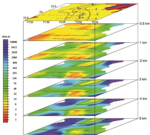
**Figure 4.** The depth slices (depths are given at the left side of each slice) obtained from inversion models are shown here. The geological map of the four profiles is marked on the top side. The letters a, b, c, d and e indicate Sanchore depression, Tharad ridge, Diyodar ridge, Patan and Mehsana sub-basins respectively.
