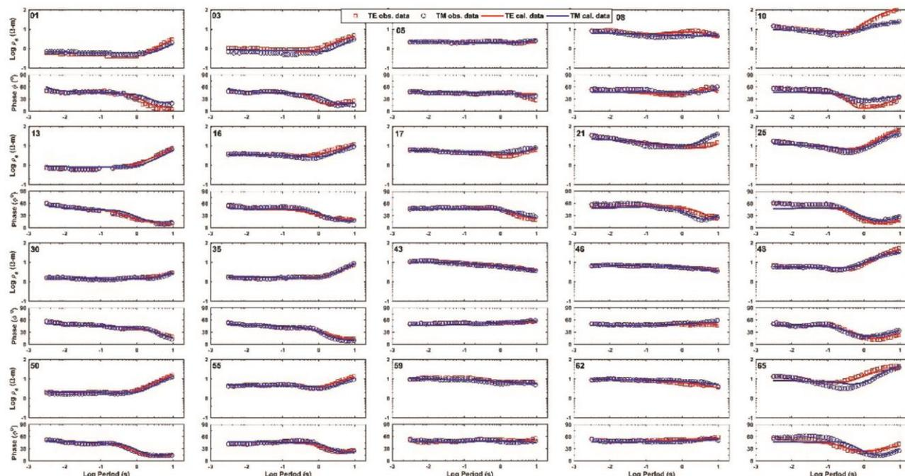
**Figure 3.** 2D inversion data fit between the observed and modelled responses for a few stations. The station numbers are given on the top left side of the resistivity plot panel.
