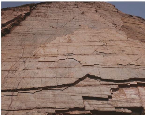
**Figure 2.** Working faces with unsafe heights and slope – a stone quarry on the outskirts of Jaipur, Rajasthan.
