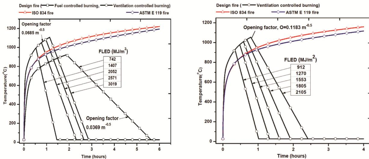
**Figure 3.** Design fire curve developed using Eurocode<sup>22</sup> for office (left) and dormitory (right) buildings.
