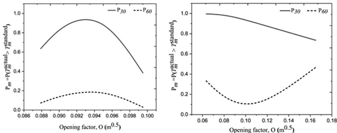
Figure 4.  $P_{30}$  and  $P_{60}$  versus opening factor for office (left) and dormitory (right) buildings.
