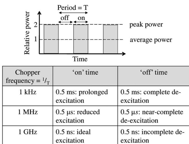
**Figure 1.** Schematic characterizing pulsed output obtained at various chopping frequencies with its effect on fluorescence.
