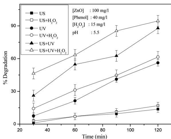
**Figure 5.** Effect of added  $\text{H}_2\text{O}_2$  on the degradation of phenol under sono-, photo- and sonophotocatalysis.
