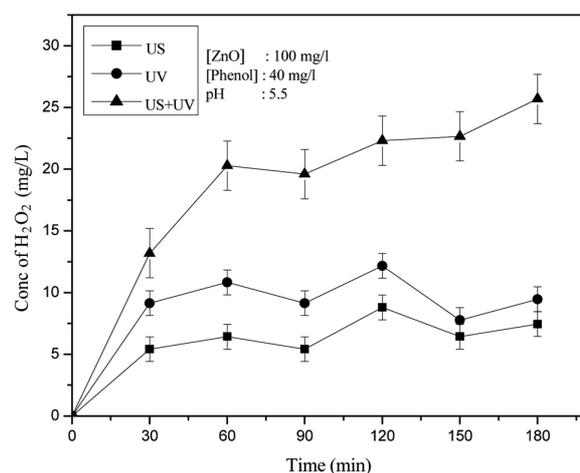
**Figure 2.** Concentration of H<sub>2</sub>O<sub>2</sub> during sono-, photo- and sonophotocatalytic degradation of phenol in the presence of ZnO.
