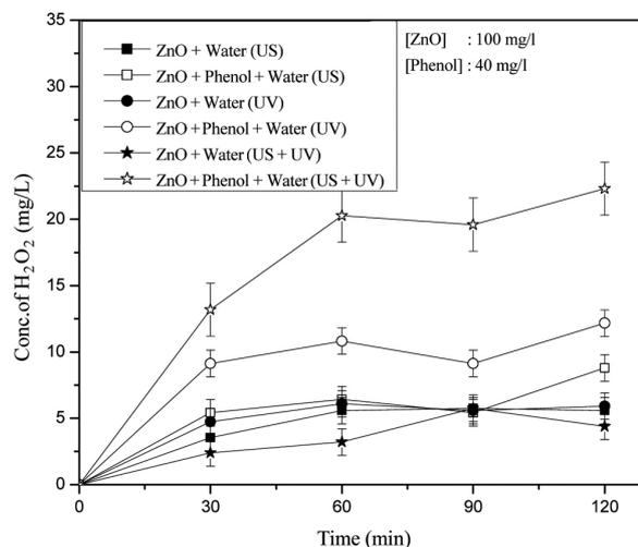
**Figure 4.** Influence of presence of phenol on net concentration of H<sub>2</sub>O<sub>2</sub> in the sono-, photo- and sonophotocatalytic system.
