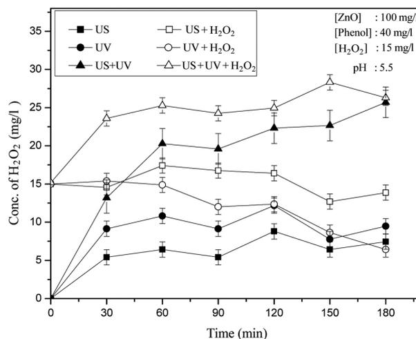
**Figure 6.** Effect of added  $\text{H}_2\text{O}_2$  on net concentration of  $\text{H}_2\text{O}_2$  under sono-, photo- and sonophotocatalysis.
