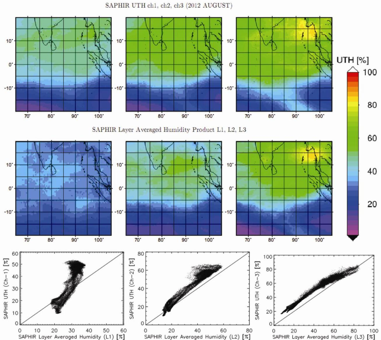
**Figure 4.** SAPHIR-UTH (top panel, channels 1–3), layer averaged humidity product from SAPHIR (middle panel, layers 1–3) for August 2012 and correlation between SAPHIR-UTH and the layer averaged humidity product from SAPHIR (bottom panel).
