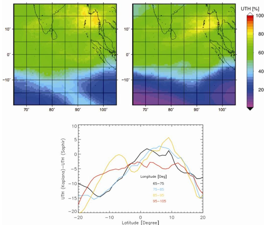
**Figure 3.** Comparison of UTH derived from SAPHIR (top, left) and the UTH product from Kalpana VHRR data (top, right). (Bottom) Latitudinal variation of the difference in UTH averaged for different longitudinal sectors.
