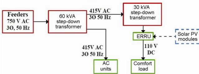
Figure 4. Power flow diagram of the existing system with proposed modifications.
