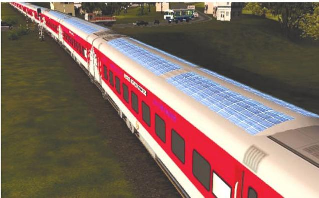
Figure 3. Graphical representation of a LHB coach mounted with solar PV modules.
