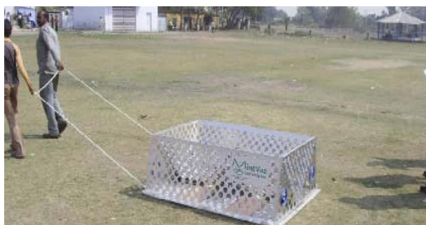
Figure 1. MineVue radar survey on the surface in coal-mining areas.
