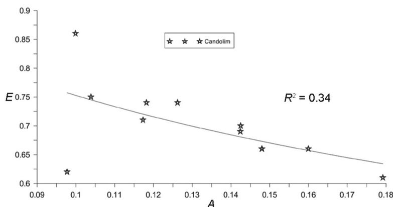
**Figure 7.** Relationship between sediment scale parameter and profile shape factor for profiles from Candolim.
