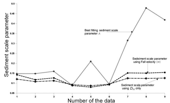
Figure 6. Dependence of sediment scale parameter  $A$  on sediment grain size and fall velocity.
