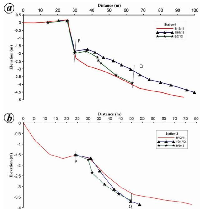
Figure 2. Beach profiles at Candolim (a) station-1 and (b) station-2.
