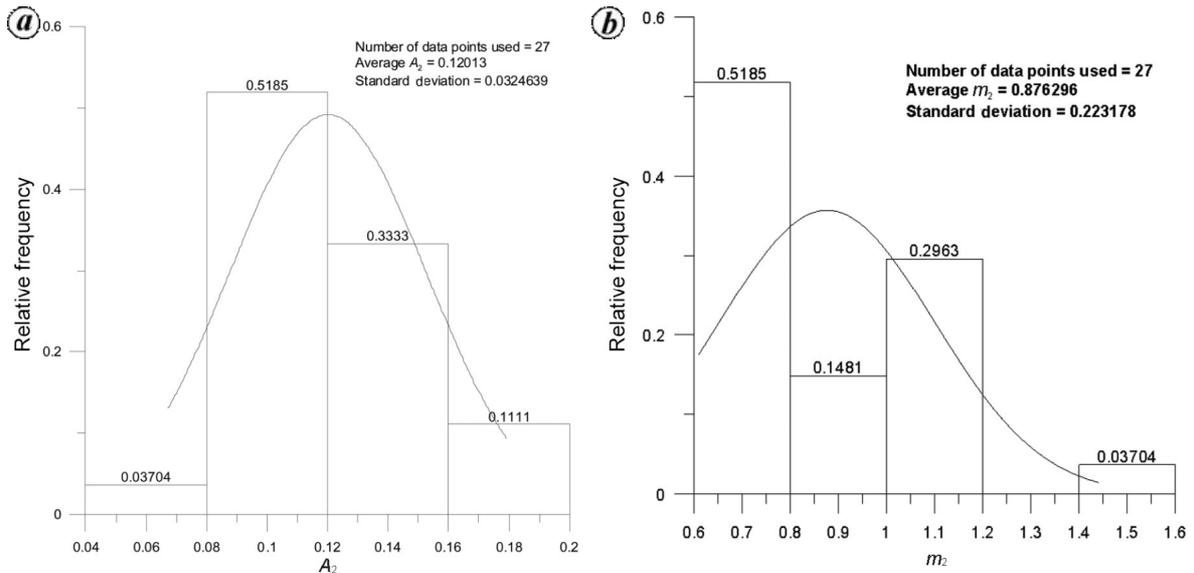
Figure 8. Histogram of best-fit values of (a)  $A_2$  and (b)  $m_2$  for nine profiles from Candolim, Miramar and Keri beaches.
