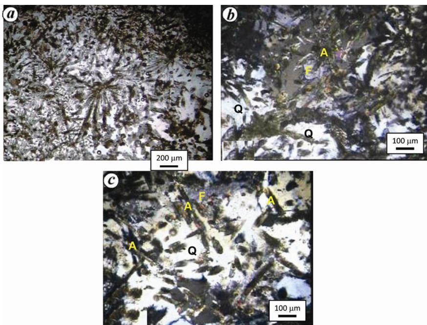
**Figure 3 a–c.** Photomicrographs of microgranite from Bhatikhera. *a*, Rosette-shaped and fine needles of aegirine in microgranite. TL – transmitted light, 1 Nicols (plane polarized light) in air. *b*, Intergrowth of coarse quartz (Q), fine feldspar (F) and needle-shaped aegirine (A). TL – transmitted light, 2 Nicols (cross Nicols) in air. *c*, Intergrowth of coarse quartz (Q), fine feldspar (F) and needle-shaped aegirine (A). TL – transmitted light, 2 Nicols (cross Nicols) in air.
