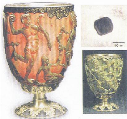
The Lycurgus Cup made of glass appears red in transmitted light and green in reflected light. The glass contains 70 nm particles as seen in the transmission electron micrograph. The cup itself is dated to 4th century AD, but the metallic holder is a later addition. (Source: <http://www.the-britishmuseum.ac.uk>.)
