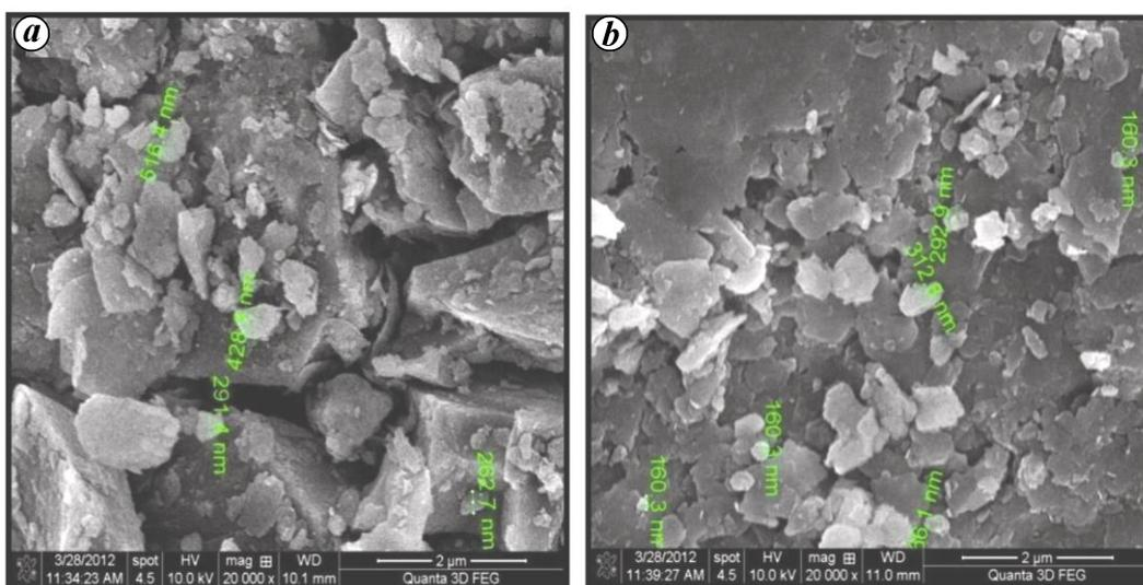
Figure 4. FESEM images of the soil sample obtained from termite hill (after grinding) for (a) sample A and (b) sample B.
