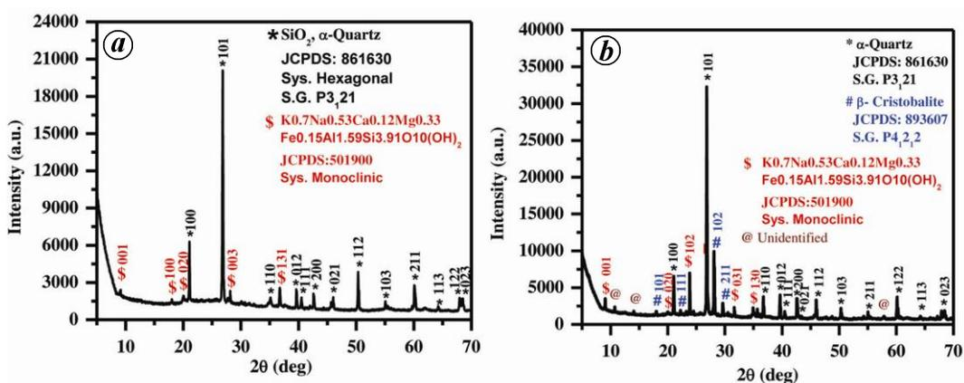
Figure 3. PXRD pattern of the soil obtained from termite hill (without grinding) for (a) sample A and (b) sample B.
