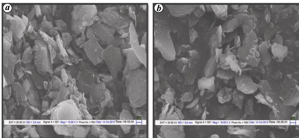
**Figure 5.** SEM images of the soil sample obtained from termite hill (without grinding) for (a) sample A and (b) sample B.
