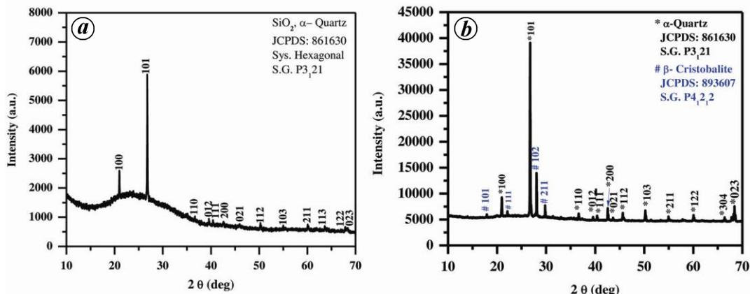
Figure 2. PXRD pattern of the soil obtained from termite hill for (a) sample A and (b) sample B.
