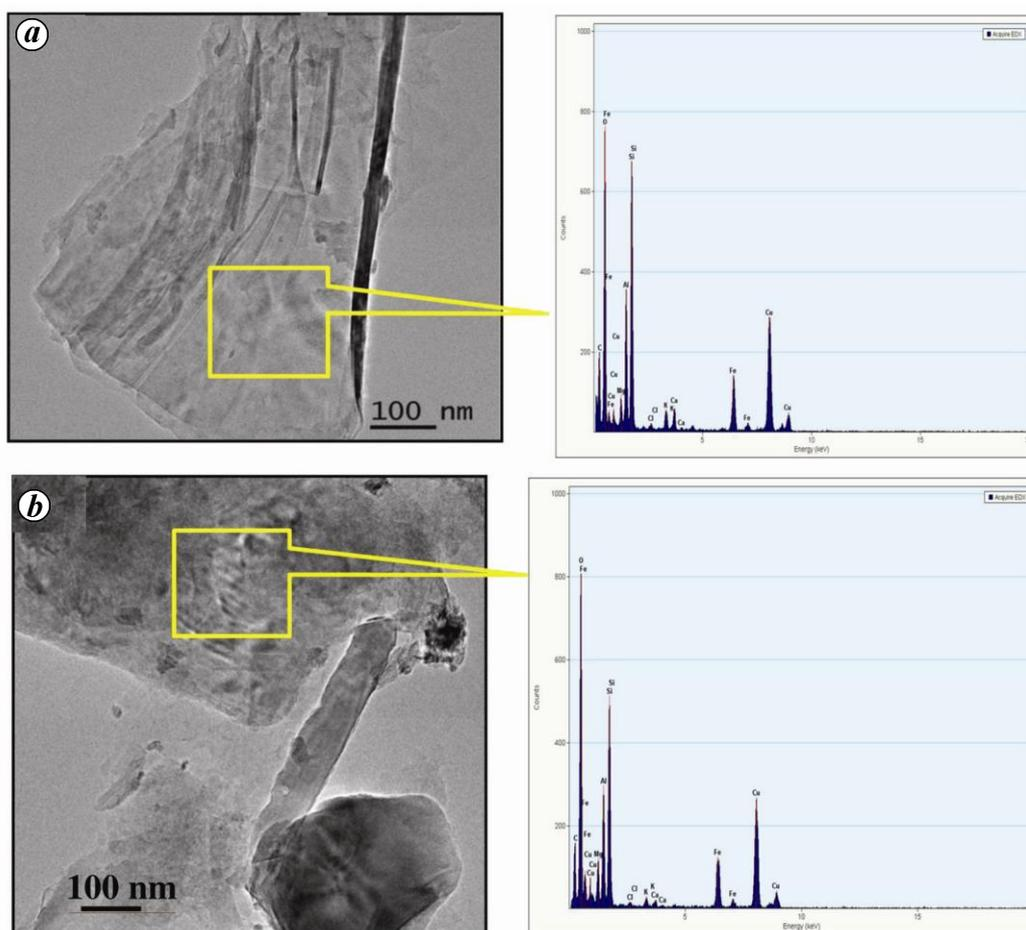
**Figure 6.** TEM images with EDAX of the soil sample obtained from termite hill for (a) sample A and (b) sample B.
