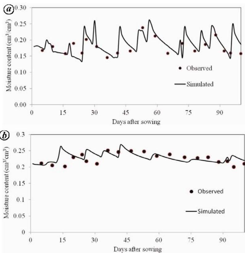
Figure 7. Model-predicted and field-observed soil moisture status for the entire crop period for pea at 30 cm depth (a) and 60 cm depth (b).
