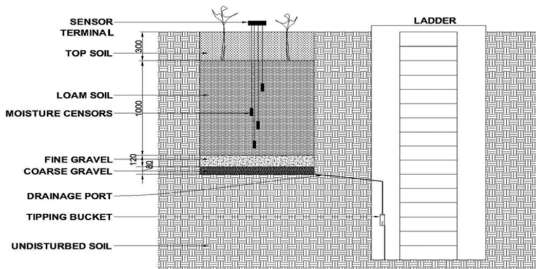
Figure 2. Lysimeter set-up.
