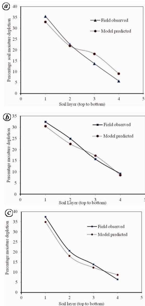
**Figure 5.** Model-predicted and field-observed soil moisture depletion for pea during the period 8–18 days after sowing (DAS) (a), 28–38 DAS (b), 46–57 DAS (c).
