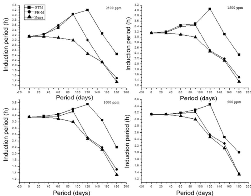
**Figure 1.** Induction period of biodiesel samples with loaded antioxidants.
