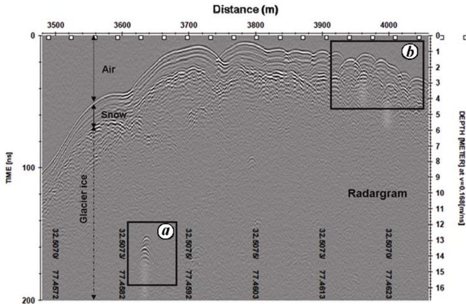
**Figure 6.** Radargram of airborne GPR profile collected from Samudra Tapu glacier *a*, Hidden crevasse, *b*, Open crevasse.
