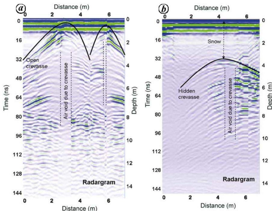
Figure 5. Radargram showing signature of open crevasse (a) and hidden crevasse (b) collected in ground mode from Siachen glacier.
