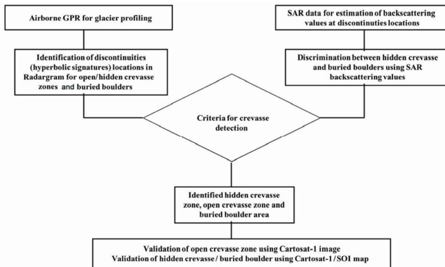
Figure 4. Flow chart of methodology for crevasse detection.
