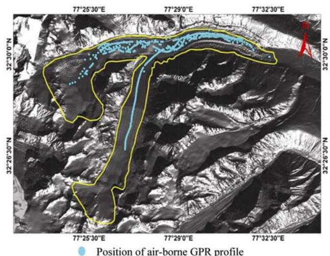
**Figure 3.** GPS points overlaid over Samudra Tapu glacier showing the positions corresponding to the airborne GPR profiles.
