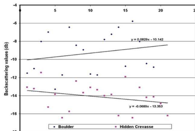
Figure 7. Backscattering values estimated using Radarsat-2 data to discriminate between hidden crevasse and buried boulders.
