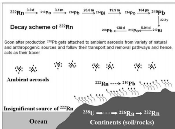
Figure 1. Schematic diagram for production and removal of  $^{210}\text{Pb}$  in the atmosphere.
