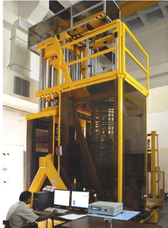
**Figure 2.** The new 1 MN force standard machine with precision digital indicator.
