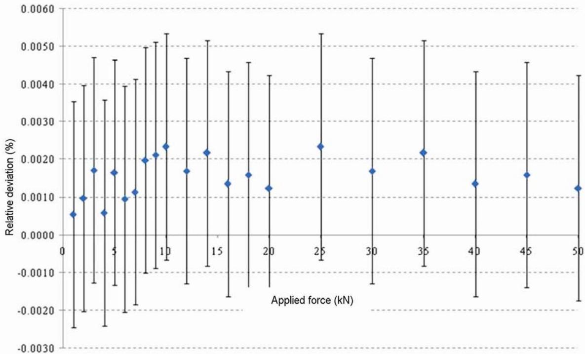
Figure 7. Relative deviation of force transducers.
