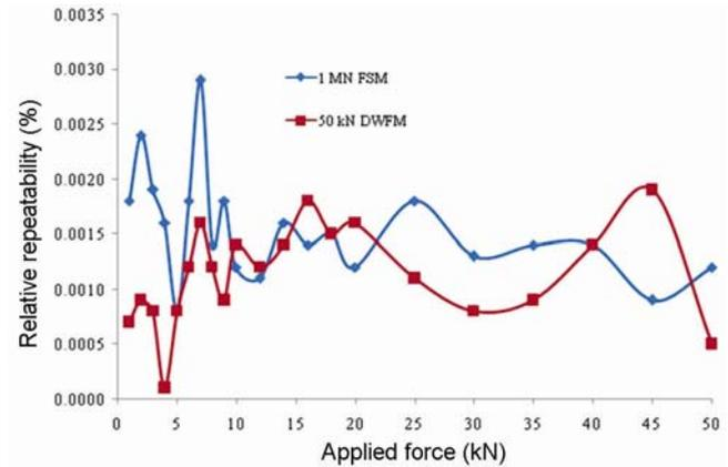
Figure 5. Relative repeatability of force transducers.
