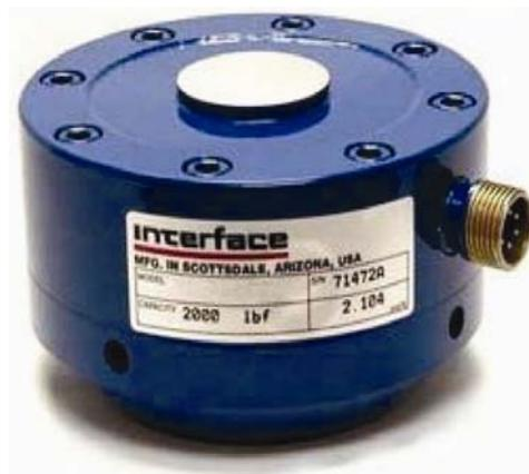
**Figure 3.** A typical precision force transducer (force transfer standard; Interface Inc. USA).
