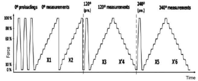
Figure 4. Schematic calibration procedure.
