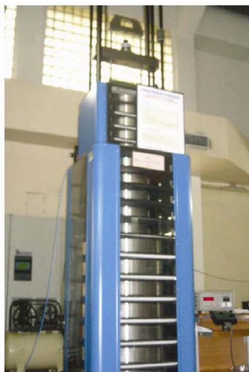
Figure 1. The 50 kN dead weight force machine.
