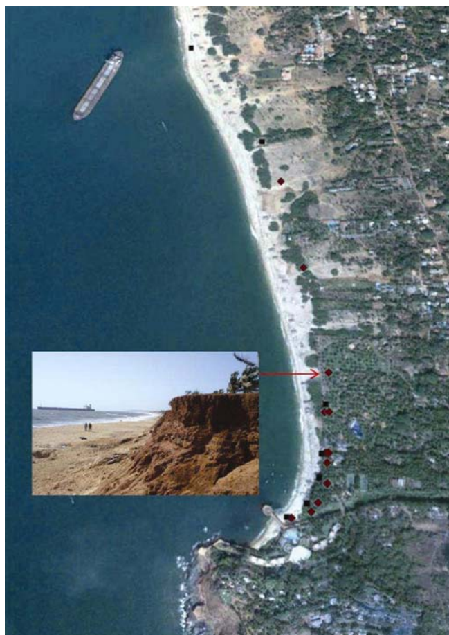
Figure 2. GPS points collected on 12 May 2008 (black squares) and 12 October 2011 (red diamonds) plotted on a Google Earth image of 5 February 2003 (courtesy: Google Earth ). (Inset) Complete elimination of a sand dune, about 4 m height, due to erosion on the Sinquerim coast (12 May 2008). The grounded super tanker MV River Princess is seen in the background.
