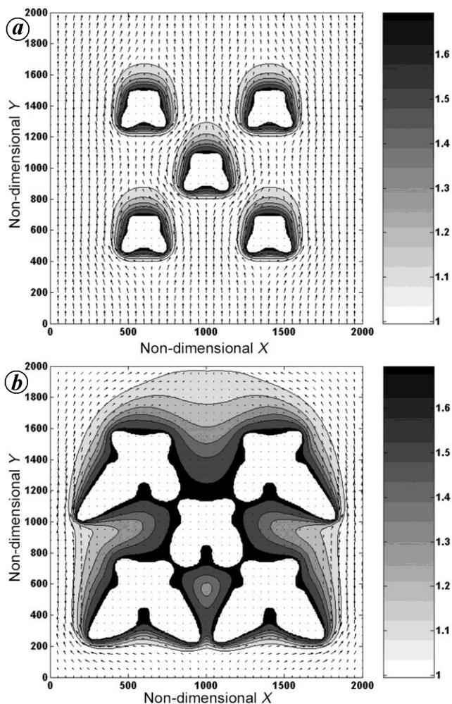
**Figure 4.** Growth pattern, concentration contours and velocity vectors for multiple dendrites evolving in a convecting melt. *a*, At non-dimensional time  $t = 6000$ ; *b*, at  $t = 20,000$ .
