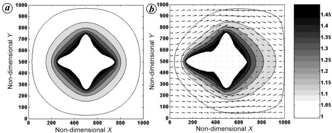
**Figure 3.** Comparison of dendrite shape and concentration contours at non-dimensional time  $t = 20,000$ . (a) Without flow and (b) with dimensionless flow velocity of  $u = 0.02$ .
