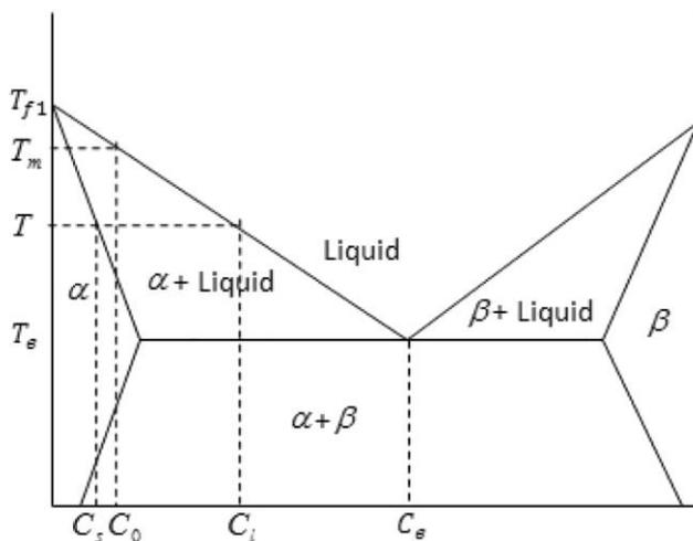
**Figure 2.** Representative phase diagram for a binary alloy.
