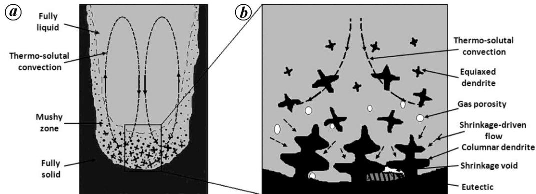
**Figure 1.** Schematic diagram showing various system-scale and micro-scale phenomena occurring during a typical casting process.
