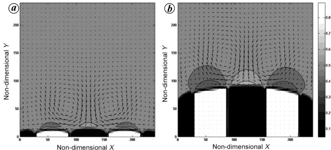
**Figure 6.** Eutectic front position, velocity vectors and concentration contours: *a*, At  $t = 4000$ ; *b*, at  $t = 32,000$ .
