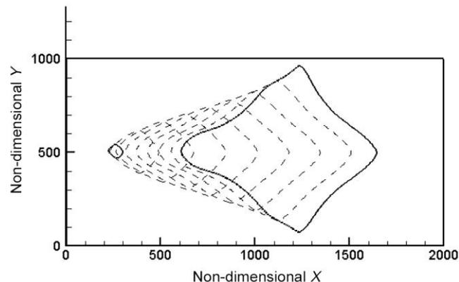
**Figure 5.** Growth and movement of dendrite in a convecting melt with  $u = 0.005$ .
