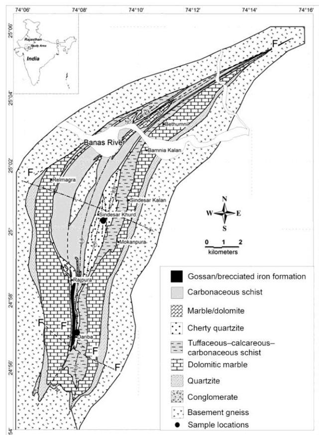
**Figure 1.** Geological map of the Dariba–Rajpura–Bethumni belt showing important prospects and deposits and the extensive chert-bearing units in the footwall (modified after ref. 20).
