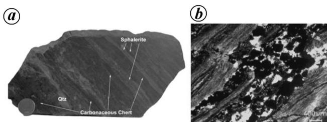
**Figure 2.** a, Fine rhythmic lamination of carbonaceous chert and sphalerite-pyrite. b, Bands of coarse-grained recrystallized ores inter-layered with fine-grained ore–quartz–carbonaceous matter association in the carbonaceous cherts.
