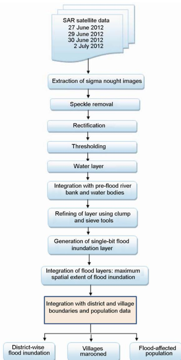
**Figure 2.** Flowchart of the methodology adopted for satellite data analysis, generation of flood inundation layer.
