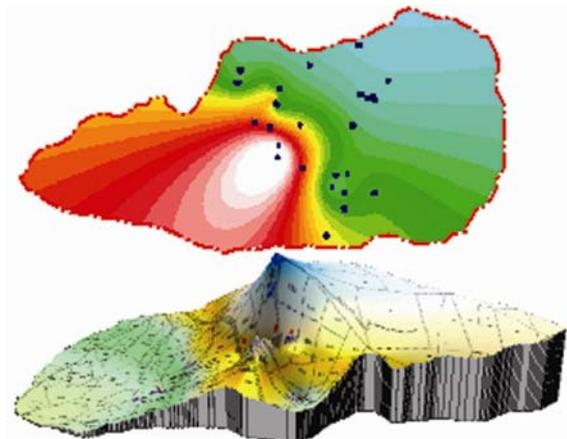
**Figure 5.** Isometric view of difference in water-table-level grids due to WHS.
