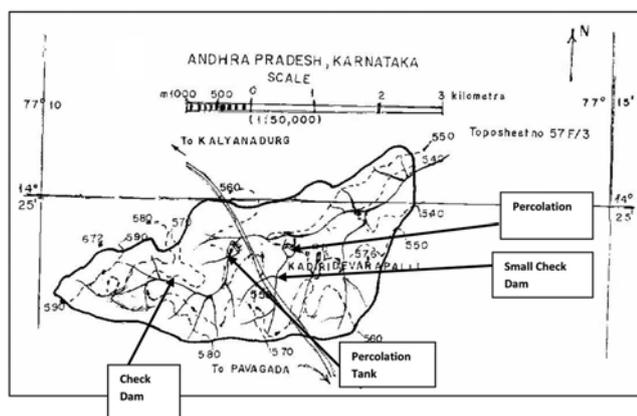
**Figure 2.** Watershed (contour map) delineated from the toposheet map showing latitude, longitude, altitude amsl and location of the water harvesting structures.
