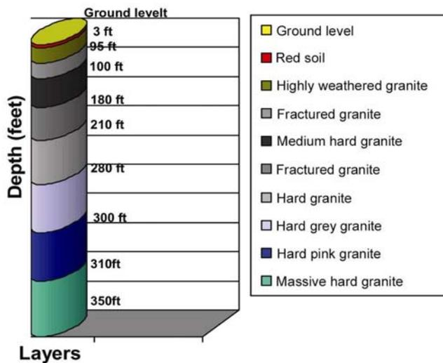
**Figure 4.** Lithological log of bore well at K. D. Pally.
