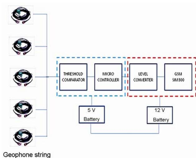
**Figure 3.** Block diagram of the proposed system model.
