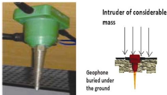
**Figure 4.** Geophone and buried geophone under the ground.
